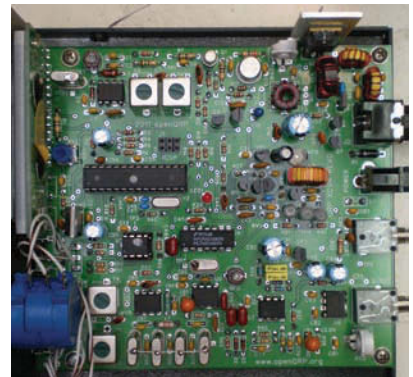
Figure 6 This low-cost, low-power continuous-wave transceiver uses a classic analog radio with a flexible programmable-control interface.
