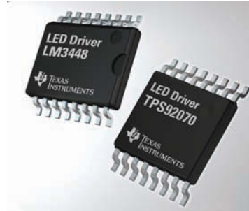
The highly integrated LM3448 and TPS92070 LED-driver ICs ease design complexity.
